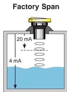
**E. Maximum Applied Range:** The Individual or cumulative effects of agitation, vapor or foam can reduce the overall quality of signal return and shorten the maximum applied range of the transmitter. To determine the maximum applied range of the transmitter in your application, refer to the below derating chart.
