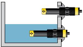
Always install the 3/4" Viton gasket with the metric (long sensor length) versions of the L\_\_-\_2\_. The G threaded version of the Switch-Tek™ will not seal unless the gasket is installed properly.
