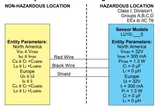
Sensor Drawing: U10900 Sheet 1 of 2 Rev. B 4-02-01
