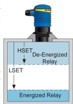
**SAF1/SAF2:** The 10A relay inside the LU30 can be used in a failsafe design of your system. When [SAF1] is set, the relay will deenergize when the acoustic return signal is LOST. When [SAF2] is set, the relay will energize when the acoustic return signal is LOST. Response times will vary according to the setting of the LU30 ([FAST] or [SLOW] modes).
