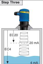
**EC4:** The 4 mA setting for the LU30. The EC4 is the distance from the bottom of the LU30 to the 4 mA set point. This setting is measured in either inches or centimeters on the display. The EC4 setting is typically greater that the EC20 setting.
