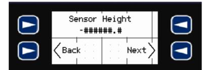
11. To change the **Sensor Height** value, first press the **ENTER** key. The value will now be highlighted and you can enter the number using the **F-Keys** as you would a 10-digit key pad, with the down arrow to enter the decimal point. Then, press **ENTER** again to complete the entry and store the value into memory.
