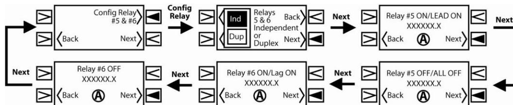
**Ⓐ Press ENTER to begin, using the F1 through F10 buttons to enter the number and press ENTER again to save the value.**
