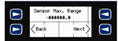
5. To change the **Sensor Max. Range** value, first press the **ENTER** key. The value will now be highlighted and you can enter the number using the **F-Keys** as you would a 10-digit key pad, with the down arrow to enter the decimal point. Then, press **ENTER** again to complete the entry and store the value into memory.
