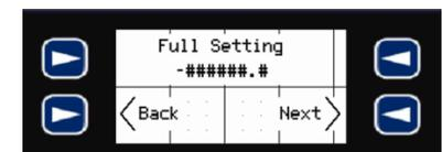
20. Press the **Next Soft Key** to return to the **Config Inputs** and **Config Outputs** screen.
