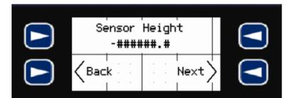
10. To change the **Sensor Height** value, first press the **ENTER** key. The value will now be highlighted and you can enter the number using the **F-Keys** as you would a 10-digit key pad, with the down arrow to enter the decimal point. Then, press **ENTER** again to complete the entry and store the value into memory.
