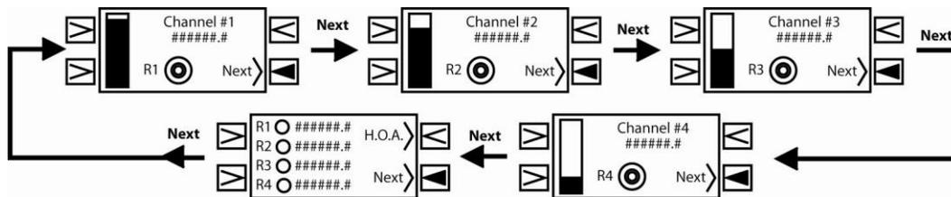
The Opening Screen indicates the Level of Liquid in the tank/vessel, along with the true analog (4-20 mA) for channel #1 and the status of Relay #1. Regardless on how the channel's level is configured the bar graph will show the true 4-20 mA level provided by the sensor.
