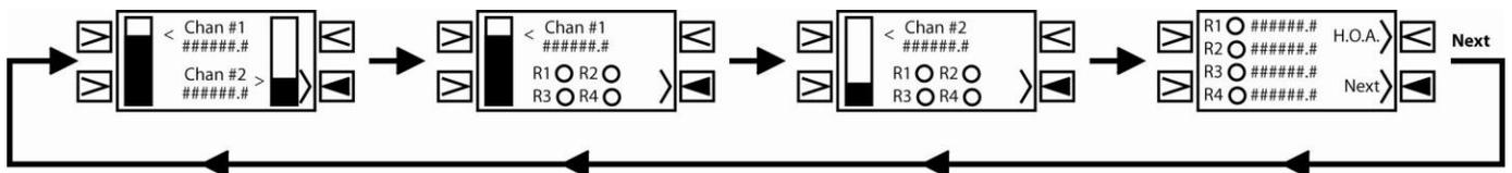
The Opening Screen indicates the Level of Liquid in the tank/vessel, along with the true analog data (4-20 mA) for channels #1 and #2. Regardless on how the channel's level is configured the bar graph will show the true 4-20 mA level provided by the sensor.
