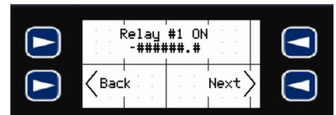
now be highlighted and you can enter the number using the **F-Keys** as you would a 10-digit key pad, with the down arrow to enter the decimal point. Then, press **ENTER** again to complete the entry and store the value into memory.
