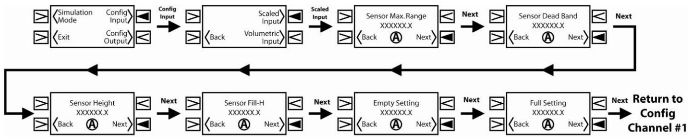
**A** Press ENTER to begin, using the F1 through F10 buttons to enter the number and press ENTER again to save the value.
