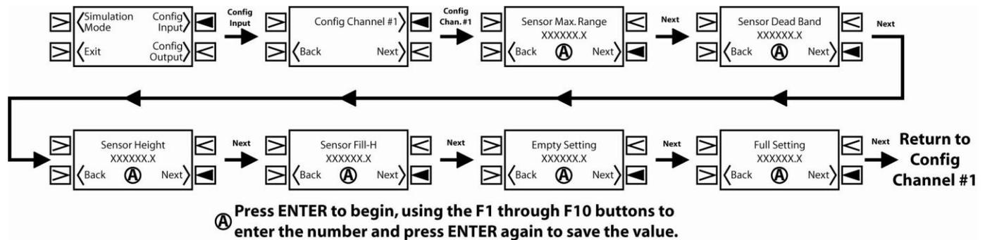
2. Press the **Config Inputs Soft Key** to begin. The first screen to appear is for Channel #1.
