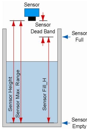
**Sensor with Non-Scaled Output (fixed output)**
