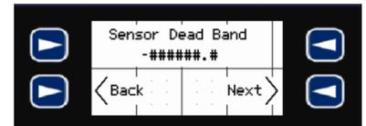
7. To change the **Sensor Dead Band** value, first press the **ENTER** key. The value will now be highlighted and you can enter the number using the **F-Keys** as you would a 10-digit key pad, with the down arrow to enter the decimal point. Then, press **ENTER** again to complete the entry and store the value into memory.
