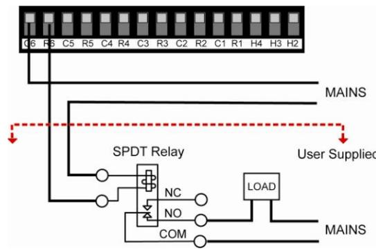
Relay wiring example
