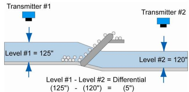
**EXAMPLE:** Relay #3 will energize when the difference between Level #1 and Level #2 is greater than 35". Relay #3 will de-energize when the difference between Level #1 and Level #2 is less than 10". Level #1 is the upstream level used for main differential control while Level #2 is the downstream level.
