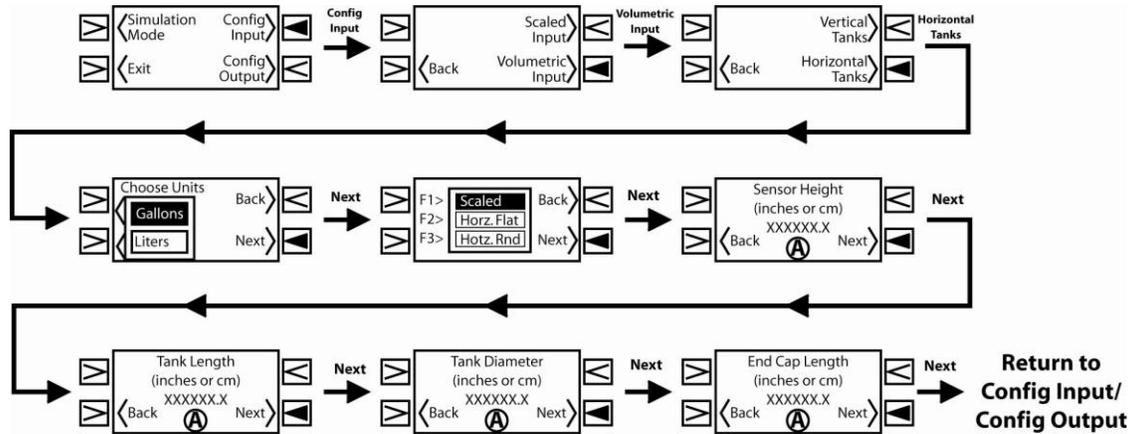
Press ENTER to begin, using the F1 through F10 buttons to enter the number and press ENTER again to save the value.
