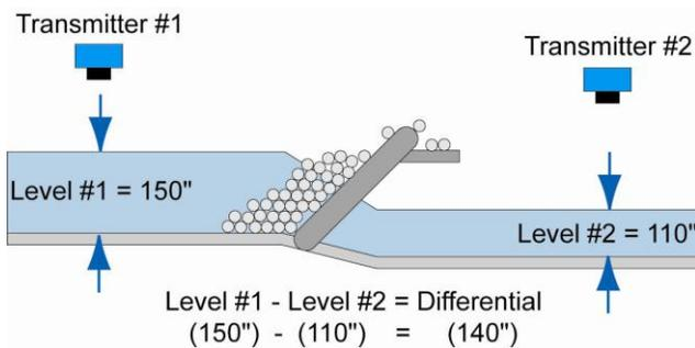
Differential less than 10", Relay #3 will de-energize
