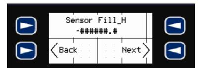
13. To change the **Sensor Fill-H** value, first press the **ENTER** key. The value will now be highlighted and you can enter the number using the **F-Keys** as you would a 10-digit key pad, with the down arrow to enter the decimal point. Then, press **ENTER** again to complete the entry and store the value into memory.
