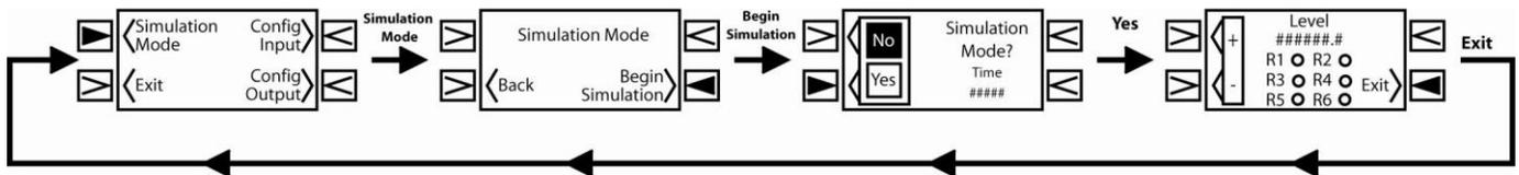
2. Press the **Simulation Mode Soft Key** to begin. The first screen to appear is for **Simulation Mode**.
