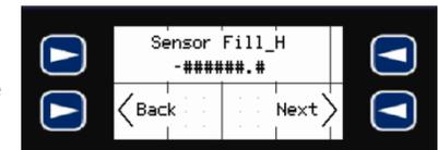
14. To change the **Sensor Fill-H** value, first press the **ENTER** key. The value will now be highlighted and you can enter the number using the **F-Keys** as you would a 10-digit key pad, with the down arrow to enter the decimal point. Then, press **ENTER** again to complete the entry and store the value into memory.
