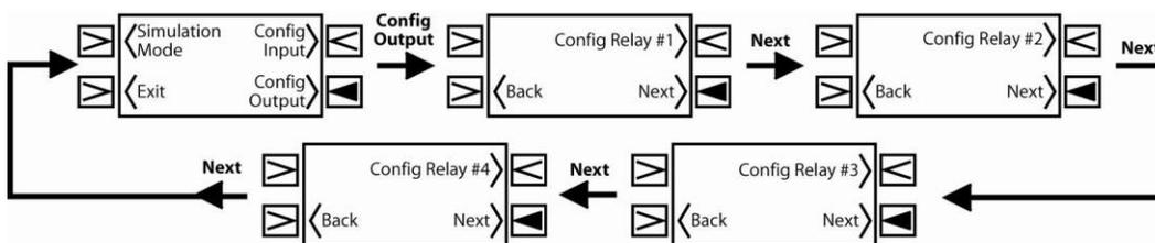
To configure outgoing data, simply press the Config Outputs Soft Key from within the Secured Functions section. Press the Next or Back soft keys to scroll to the area you would like to configure. The above illustration is for a 4 output configuration. Configurations with a different number of relay outputs will differ slightly.
