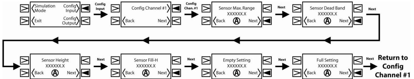
**A** Press ENTER to begin, using the F1 through F10 buttons to enter the number and press ENTER again to save the value.
