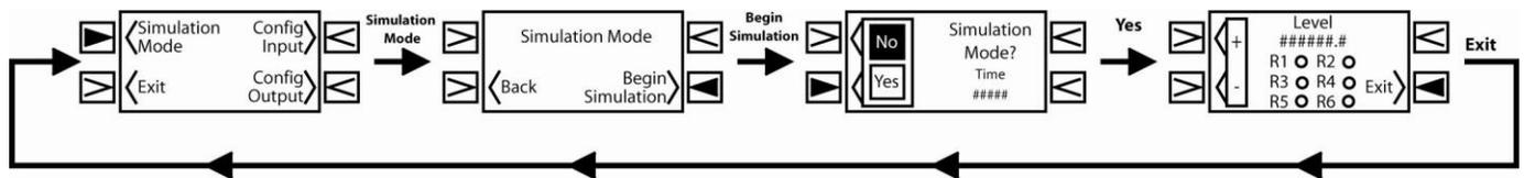
Simulation Mode allows users to simulate changes in tank levels. Relays will turn ON and OFF depending on how they were configured. This will test your configuration and setup. The above illustration is for a 1 input configuration. Configurations with a different number of inputs will differ slightly.
