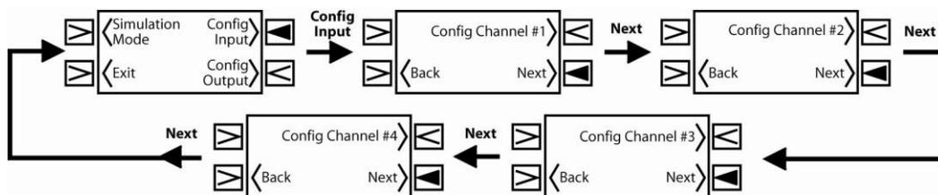
To configure sensor inputs, simply press the Config Inputs Soft Key from within the Secured Functions section. Press the Next or Back soft keys to scroll to the area you would like to configure. The above illustration is for a 4 input configuration. Configurations with a different number of inputs will differ slightly.
