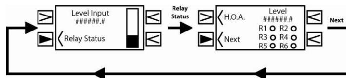
The Opening Screen indicates the Level of Liquid in the tank/vessel, along with the true analog data (4-20 mA) for channels #1. Regardless how the channel's level is configured the bar graph will show the true 4-20 mA level provided by the sensor.
