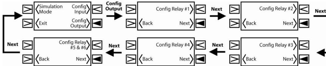
To configure outgoing data, simply press the Config Outputs Soft Key from within the Secured Functions section. Press the Next or Back soft keys to scroll to the relay you would like to configure. As an option, Relays 5 and 6 can be used as a Duplex / Alternation function. Select the Config. Relay #5 and #6 upper right soft key to configure relays #5 and #6. This setting will always configure both relays #5 and #6.
