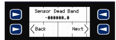
8. To change the **Sensor Dead Band** value, first press the **ENTER** key. The value will now be highlighted and you can enter the number using the **F-Keys** as you would a 10-digit key pad, with the down arrow to enter the decimal point. Then, press **ENTER** again to complete the entry and store the value into memory.
