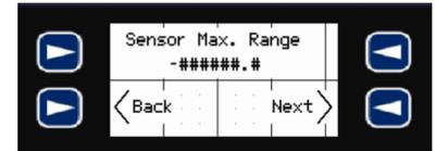
4. To change the **Sensor Max. Range** value, first press the **ENTER** key. The value will now be highlighted and you can enter the number using the **F-Keys** as you would a 10-digit key pad, with the down arrow to enter the decimal point. Then, press **ENTER** again to complete the entry and store the value into memory.
