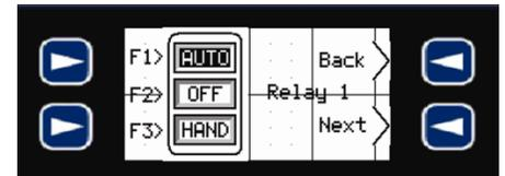
The first time the Commander Controller is powered up, all of the relays will be in the OFF mode. To activate the relay, you will need to change the relay mode to AUTO.
