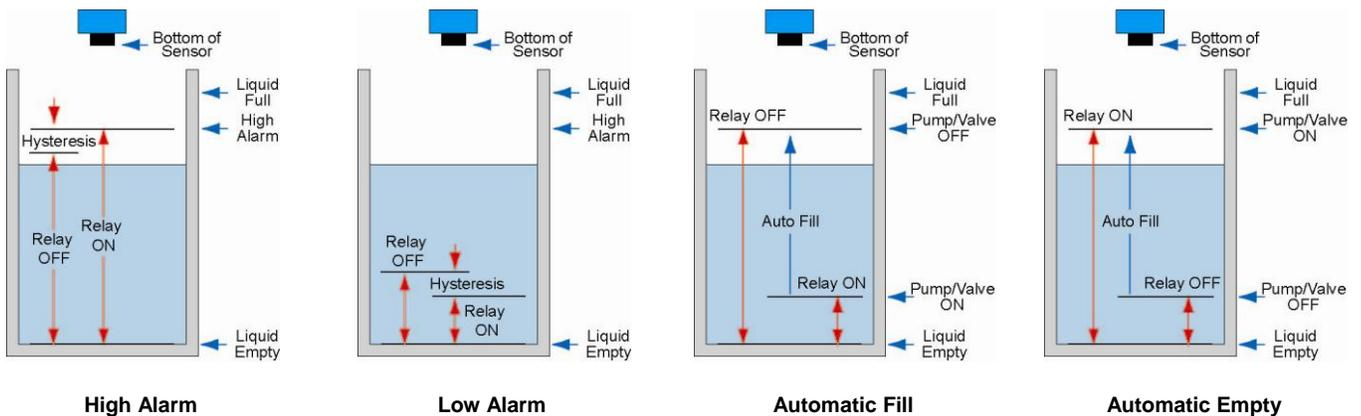
**EXAMPLE:** If a tank’s sensor is reading between 0 to 500 gallons, then the relay set points must be measured in gallons. For Alarms (High or Low), use the ON point where the relay will start and the OFF as a hysteresis to prevent chattering of the relay. For Pumps and Valves (Auto Fill or Auto Empty), use both settings as the ON/OPEN and OFF/CLOSE points for the device.
