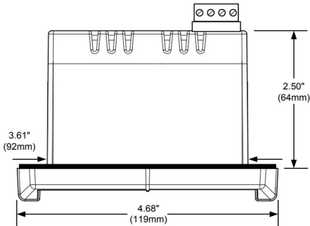
**Figure 6. Case Dimensions – Top View**
