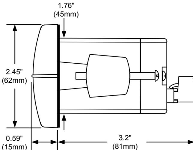
**Figure 5. Meter Dimensions – Side View**
