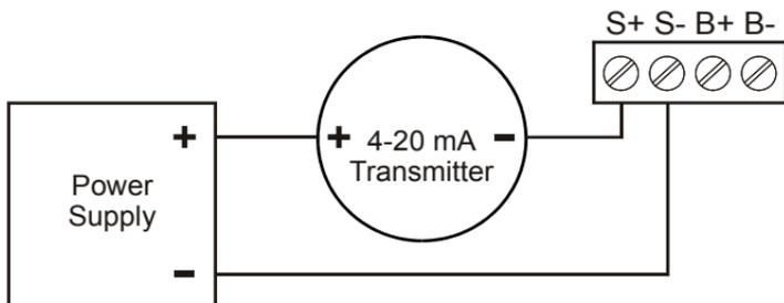
Figure 4. Input Connections without Backlight
