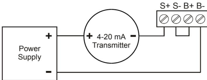
Figure 3. Input Connections with Backlight
