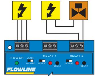
**NOTE:** If the device's load exceeds the rating of the controller's relay, a stepper relay of higher capacity must be used as part of the system design.
