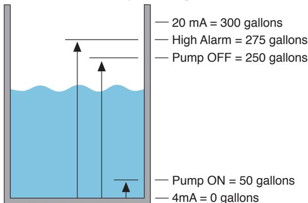
Enter all values into the LC52 in gallons. The OFFSET is the corresponding 4 mA setting in gallons. The SPAN is the corresponding 20 mA setting in gallons. RLY2A and RLY2B is dedicated to the filling of the tank because RELAY2 is a latching relay. RLY1 is dedicated to the high level alarm because it is a single set point relay. Use the following values for programming the LC52-1001.
