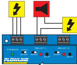
To do this, connect the hot lead of the alarm to the NC side of the relay terminal of the LC52. If
