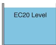
To calibrate EC20, set the tank to the new Span level. Press [20] button once and [E] will appear in the display. Press [20] button again and [C] will appear in the display and EC20 is set.
