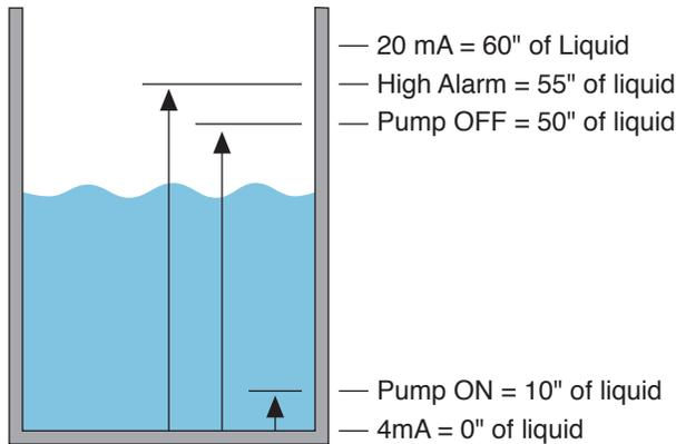
Enter all values into the LC52 in inches. The OFFSET is the corresponding 4 mA setting in inches. The SPAN is the corresponding 20 mA setting in inches. RLY2A and RLY2B is dedicated to the filling of the tank because RELAY2 is a latching relay. RLY1 is dedicated to the high level alarm because it is a single set point relay. Use the following values for programming the LC52-1001.
