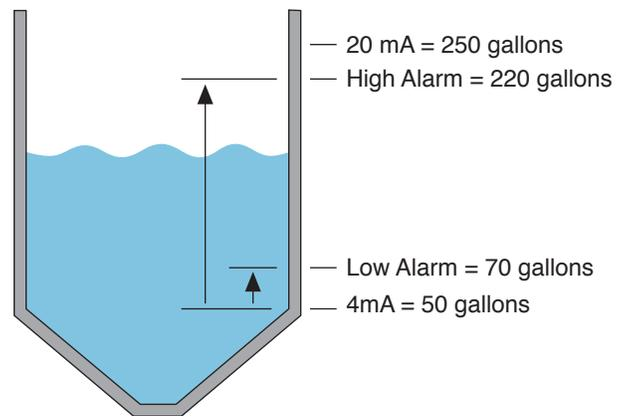
Enter all values into the LC52 in gallons. The OFFSET is the corresponding 4 mA setting in gallons. The SPAN is the corresponding 20 mA setting in gallons. RLY1 is dedicated to the high level alarm because it is a single set point relay. RLY2A is dedicated to the low level alarm because the latch is turned off on Relay 2. Use the following values for programming the LC52-1001.
