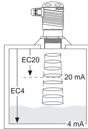
**EC4:** The 4 mA setting for the LU20. The EC4 is the distance from the bottom of the LU20 to the 4 mA set point. This setting is measured in either inches or centimeters on the display. The EC4 setting is typically greater than the EC20 setting.
