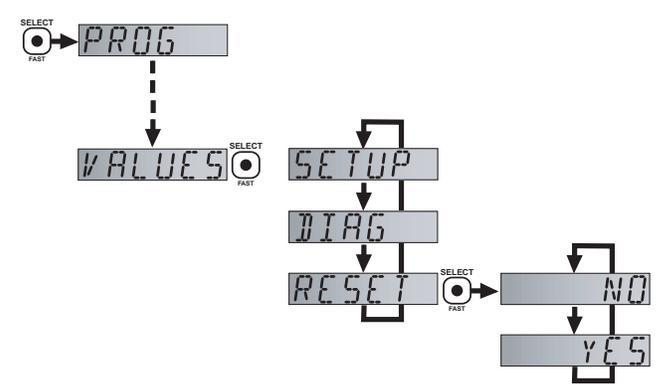
1. Press the SELECT/FAST button and hold it for 5 seconds until PROG appears.
