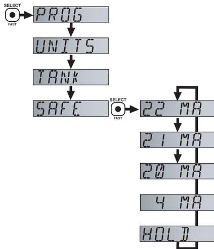
1. Press the SELECT/FAST button and hold it for 5 seconds until PROG appears.
