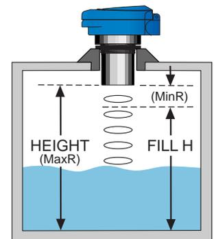
**K. REV mA (Reverse mA):** Allows the user to select 20 mA at the bottom and 4 mA at the top of the tank (20-4 mA). Factory default is 4 mA (MaxR) at the bottom and 20 mA (MinR) at the top.
