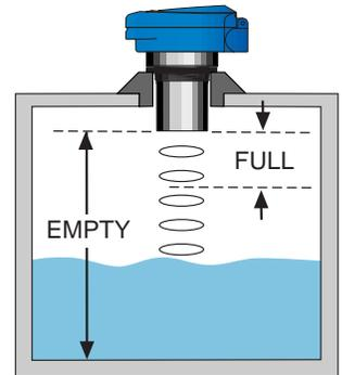
**J. Fill H (Fill Height):** The point in inches or centimeters from the bottom of the tank to the high level where the output will be 20 mA (generally the straight wall distance from the bottom of the tank). NOTE: The transmitter dead band is automatically subtracted from the FILL H. Example: LU81 = 4" dead band. Therefore the maximum FILL H is 197" [maximum range] - 4" [dead band] = 193".
