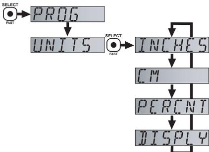
1. Press the SELECT/FAST button and hold it for 5 seconds until PROG appears.
