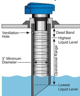
**A. Fitting Selection:** Check the transmitter part number to determine the required 2" fitting thread type. The transmitter is commonly installed in tank adapters, flanges, brackets or stand pipes.
