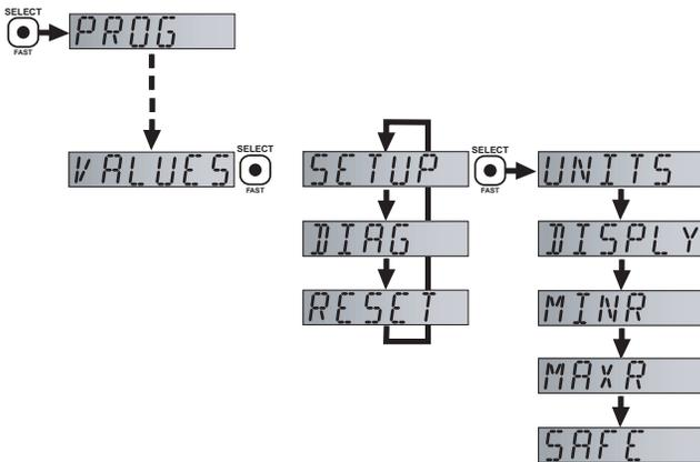
1. Press the SELECT/FAST button and hold it for 5 seconds until PROG appears.
