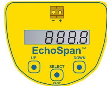
**B. Entering the Program Mode:** Press and hold the SELECT/FAST button for approximately 5 seconds until the display changes from a numeric value to PROG, indicating that you have entered the PROG mode.
