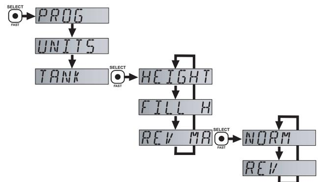
**NOTE:** You must set HEIGHT and FULL R prior to reversing the 4 and 20 mA. Regardless of which mode you are in (Norm or Rev), changes to the HEIGHT or FULL R are always with respect to the original settings programmed.
