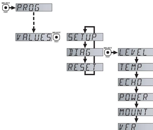
1. Press the SELECT/FAST button and hold it for 5 seconds until PROG appears.
