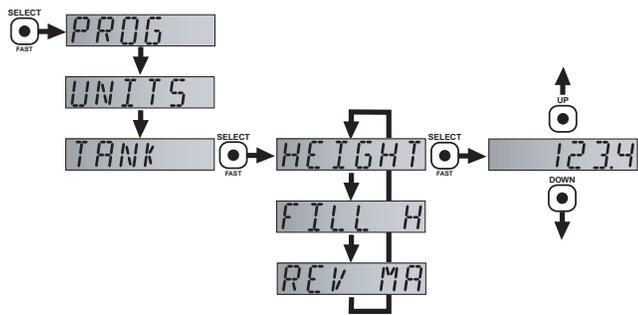
1. Press the SELECT/FAST button and hold it for 5 seconds until PROG appears.
