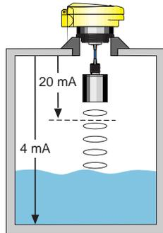
**D. Maximum Applied Range:** The Individual or cumulative effects of agitation, vapor or foam can reduce the overall quality of signal return and shorten the maximum applied range of the transmitter. To determine the maximum applied range of the transmitter in your application, refer to the below derating chart.
