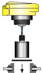
**A. Fitting Selection:** The transmitter is commonly installed in tank adapters, flanges, brackets or stand pipes.
