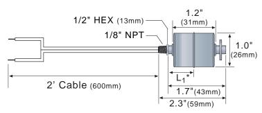
$L_1^* = 0.6$ " (15mm) NO, .8" (21mm) NO, switch actuation level, nominal (based upon specific gravity = 1.0)
