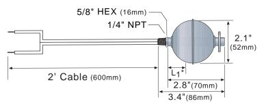
$L_1^* = 1.1$ " (28mm) NO, dimension varies for NC switch actuation level, nominal (based upon specific gravity = 1.0)
