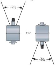
Normally Open or Normally Closed: Each level switch can be wired Normally Open (NO) or Normally Closed (NC). The Normal Condition is typically when the float rests in a dry state. Each LV30 series level switch is shipped in the NO state and can be switched in the field by rotating the float 180 degrees. The float is marked NO or NC along the side to easily indicate the state of the switch.
