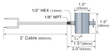
$L_1^* = 0.6$ " (16mm) NO, .8" (19mm) NO, switch actuation level, nominal (based upon specific gravity = 1.0)
