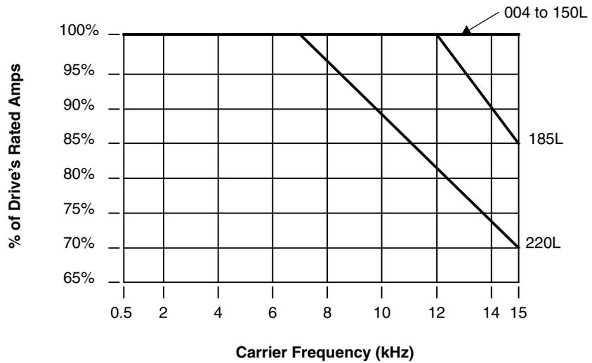
**SJ300 30 to 55 kW at 50 deg. C ambient**
