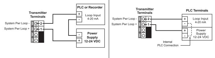
Example: Two transmitters connected to PLC/Recorder with separate power supply
