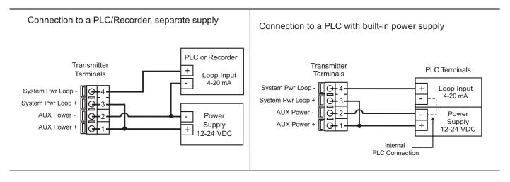
Two transmitters connected to PLC/Recorder with separate power supply
