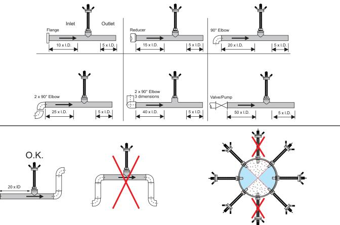
Located the magmeter in a "trap" to prevent air bubbles and to keep the electrodes wetted for best performance.
