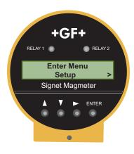
Use the keypad to navigate through each setting.
