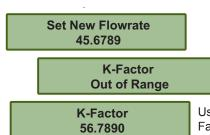
The flow rate shown is based on the existing calibration of the 2551. Use the keypad to modify the flow rate to match the reference meter. The 2551 will automatically calculate a new K-cactor based on the new flow rate.
