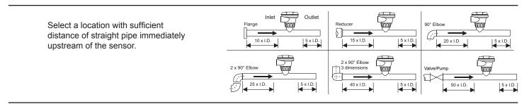
Locating the sensor in a trap or where the flow is upward helps to protect the sensor from exposure to air bubbles when the system is in operation.
