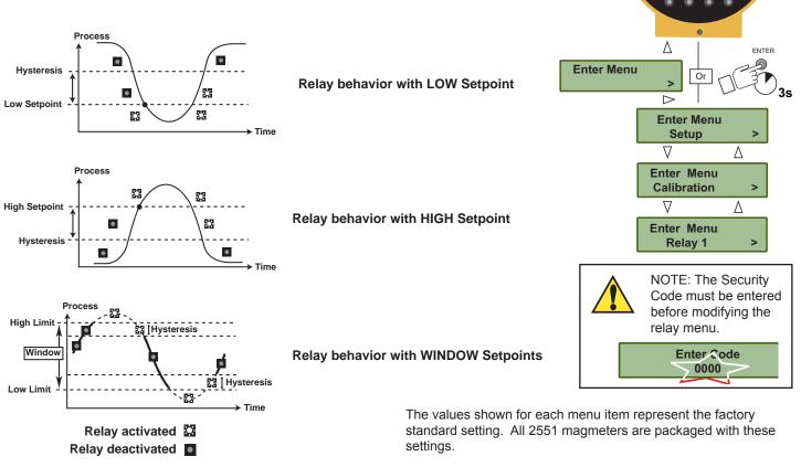
Set Low: Set the flow rate where a Low relay will be activated.
