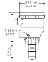
Pipe Range 1/2 to 4 in. -XO = 58 mm (2.3 in.) -X1 = 91 mm (3.6 in.) 5 to 8 in. 10 to 12 in. -X2 = 167 mm (6.6 in.)
