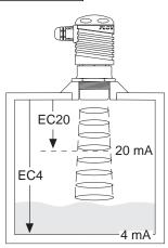
**EC4:** The 4 mA setting for the LU20. The EC4 is the distance from the bottom of the LU20 to the 4 mA set point. This setting is measured in either inches or centimeters on the display. The EC4 setting is typically greater that the EC20 setting.
