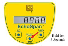
After entering the PROG mode, the display will scroll through the top menu, alternately flashing UNITS, TANK, SAFE, TG CAL, VALUES, HELP and RUN.
