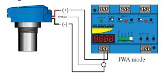
B. Wiring to a Typical Two-Wire Loop Powered Indicator
