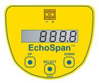
**B. Entering the Program Mode:** Press and hold the SELECT/FAST button for approximately 5 seconds until the display changes from a numeric value to PROG, indicating that you have entered the PROG mode.
