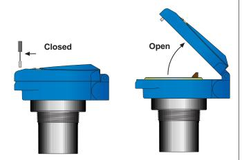
Before closing the enclosure, make sure that the enclosure gasket is properly seated, and that any conduit fittings, liquid tight cable connectors and/or plugs are properly installed and sealed.
