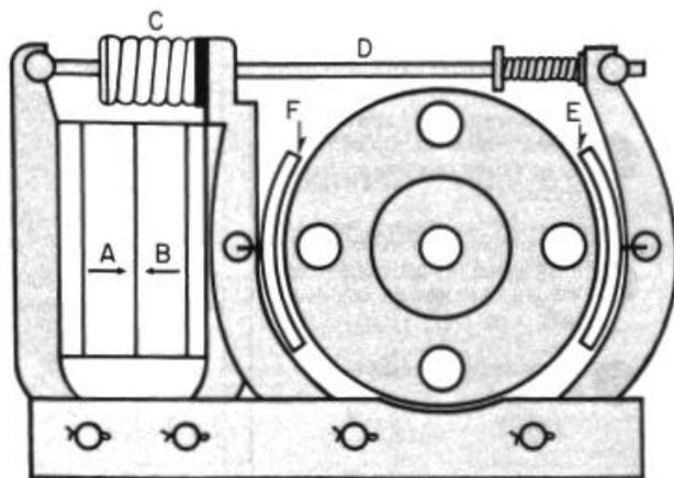
When the twin magnets (A and B) are energized, they pull together compressing spring C. This action simultaneously moves tie rod D to the right freeing shoe E. At the same instant, the motion of magnet B to the left frees shoe F.
