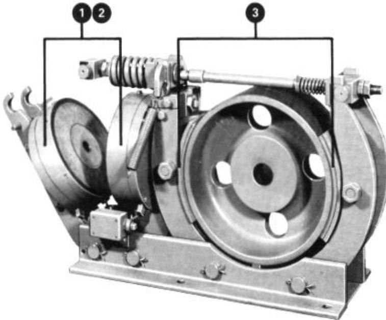
**1** Mechanically independent coils can be removed without releasing the brake shoes. The design of the twin-magnet system results in a real safety feature: if the magnet coil should need replacement while the equipment is under load, for example, while a crane is in the middle of a lift, the magnetic assembly can be removed and replaced or repaired without releasing the braking action or disturbing the torque setting. In an emergency, short-time operation on a single coil is possible.
