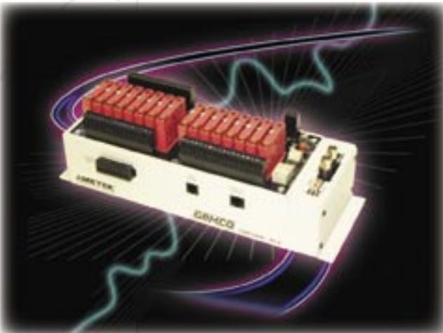
The Series 7500 incorporates Gemco's patented ULTRA HIGH SPEED technology. Of the unit's 32 total outputs, 16 operate at 5 microsecond scan times and are designed for the highest speed applications like adhesive system control. The remaining 16 outputs are ideal for the numerous lower speed applications that consume valuable I/O and processor time in the PLC.
