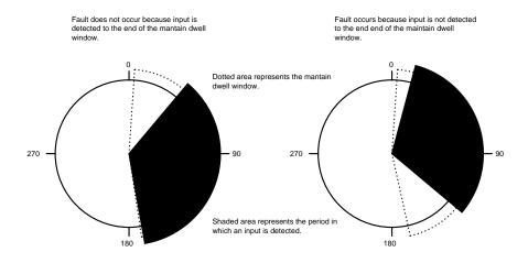
Figure 11-3 Proximity Switch Monitoring for Short Feeds
