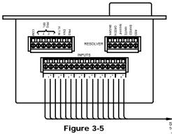
The 2500 has eight inputs that are internally tied to the eight outputs. The input connector is a sixteen position connector. Each input can be configured as either a reset-to-preset, an output enabler input or a die protection input. Inputs 1 - 8 require a PNP sourcing device type input signal.
