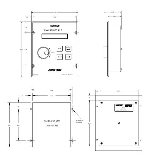
Figure 2-13: 2500R Remote Operator Interface
