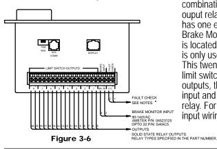
The Main Controller and Expansion Modules are available with any combination of solid-state AC or DC ouput relays. The Main Controller has one extra optional solid-state Brake Monitor input relay. This relay is located in the far left relay slot and is only used for brake monitoring. This twenty-place connector contains limit switch 1 - 8 solid-state relay outputs, the optional Brake Monitor input and the Fault Check output relay. For output or brake monitor input wiring, see Fig. 3-13 & 3-14.
