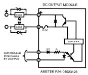
OPTO 22 P/N: G4ODC5 \* COMMUTATION DIODE MUST BE USED ON INDUCTIVE LOADS. TYPICALLY, USE DIODE IN400
