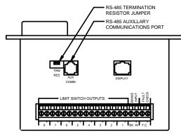
The auxillary RS485 communication port uses a standard RJ11 connector. The communication port has not been defined at this time, consult factory.
