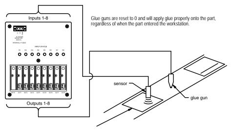
Although the part was positioned at 180 according to the resolver, the output channels' position linked to the input are reset to 0.
