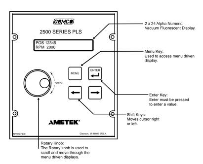
Figure 2-9: Main Controller (Front View)
