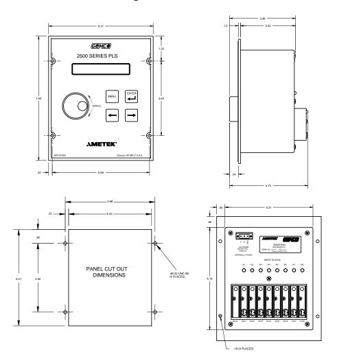
Figure 2-11: 2500CF Main Controller Dimensions
