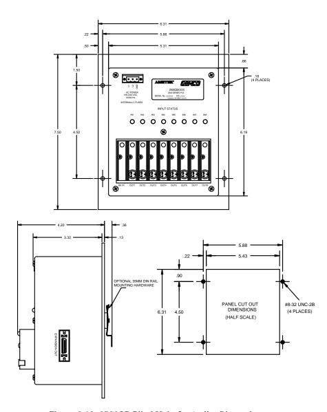
Figure 2-12: 2500CB Blind Main Controller Dimensions
