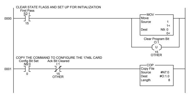
When the configuration command is complete, the program will copy the LDT configuration command for LDT 1 into the output image table with the programming bit set. This command will configure LDT 1 for the speed of wire, count direction, recirculations, and LDT length. The speed of wire for LDT 1 is  $9.300\mu s/inch$ . The counts are defined as increasing from the LDT head. There is only 1 recirculation and the LDT length is 12.0 inches. This continues until the command has been acknowledged.
